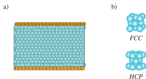
Fig. 10 (a) Example of a snapshot taken from the simulation with e_n = 0.2 , d_w = 1 and p = 2.9 \times 10^{-3} in the steady state, characterized by the presence of crystalline structures inside the flowing particles. (b) Sketch of face centered cubic (FCC) and hexagonal close pack (HCP) structures.
